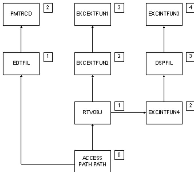
The arrows indicate the usage sequence for the functions that use the access path. The numbers in the small boxes indicate the usage level of each object relative to the access path at level 0.
